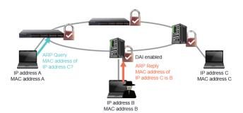
DAI validates the ARP packets in a network. DAI intercepts, logs, and discards ARP packets with invalid IP-to-MAC address bindings. This capability protects the network from some man-in-the-middle attacks.
