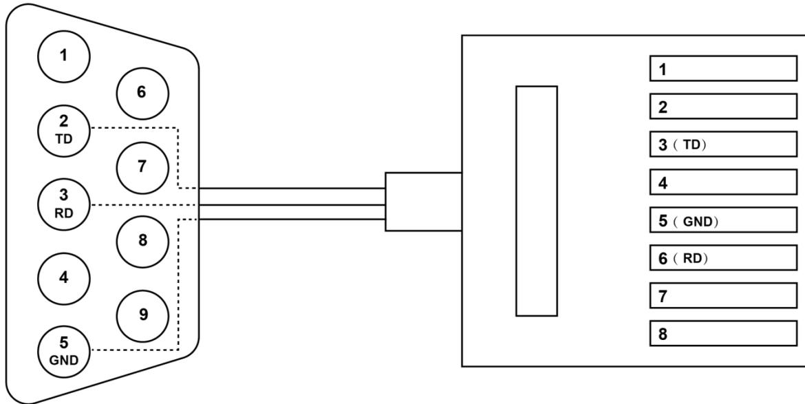
Note: We suggest to use three pin console at RJ45 end. If using 8 pin console cable at RJ45 end, please block or remove the 4th pin out.
