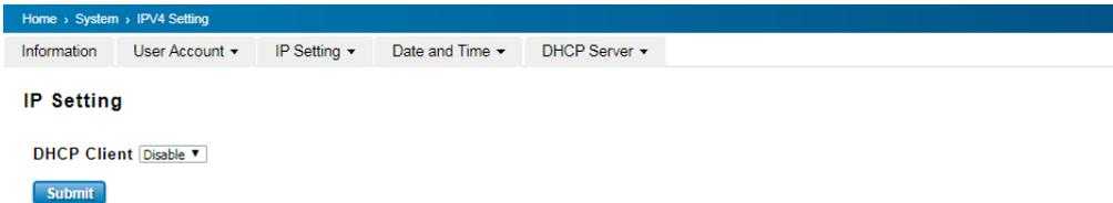
The screenshot shows a web interface for DHCP Client configuration. At the top, there is a breadcrumb trail: Home > System > IPv4 Setting. Below this, there are several tabs: Information, User Account, IP Setting (selected), Date and Time, and DHCP Server. Under the IP Setting tab, there is a section titled "IP Setting". Within this section, there is a "DHCP Client" label followed by a dropdown menu currently set to "Disable". Below the dropdown is a blue "Submit" button.
