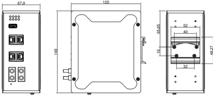
Dimensions of **6012GX4-POE** : 85.5 mm x 150 mmx 126.5 mm(W x H x D) / without DIN Rail Clip
