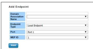
Points at the edge of the domain, define the boundary for the domain. A MEP sends and receives CFM frames through the relay function, drops all CFM frames of its level or lower that come from the wire side. All the configurations above will directly appear at the three tables below, Domain Table, Association Table and the Endpoint Table.
