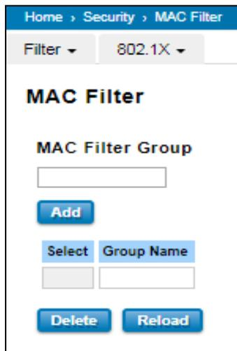
Create a group of MAC Filters by entering a name and clicking the **Add** button to create a new Filter Group. The MAC Filter Group table provides the following information. **Select** the entry and click the **Delete** button then the Filter Group is deleted. Click the **Reload** button to reload the MAC Filter Group table.
