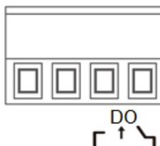
**NOTE:** The relay contact only supports 0.5 A current, DC 24V. Do not apply voltage and current higher than the specifications.
