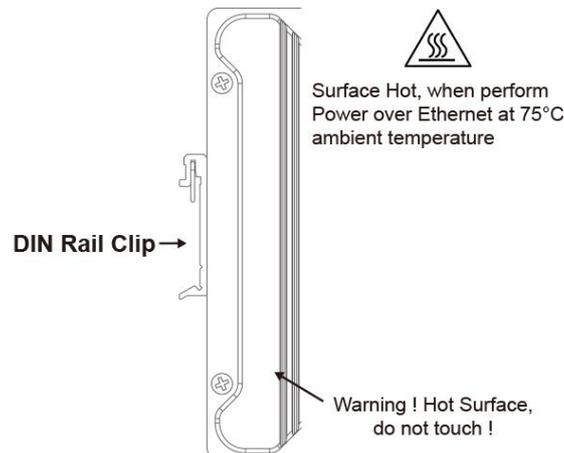
To mount the switch on DIN Rail track, do the following instruction:
