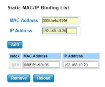
Type the specific MAC and IP address, and then click **Add** to add a new MAC & IP address binding rule for a specific client.
