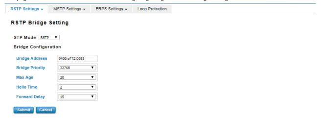
The STP mode includes the **STP**, **RSTP**, **MSTP** and **Disable**. User can select the STP mode for user system first. The default mode is RSTP enabled. After user selects the STP or RSTP mode; user should continue to configure the global Bridge parameters for STP and RSTP. If user selects the MSTP mode, user need go to MSTP Configuration page.
