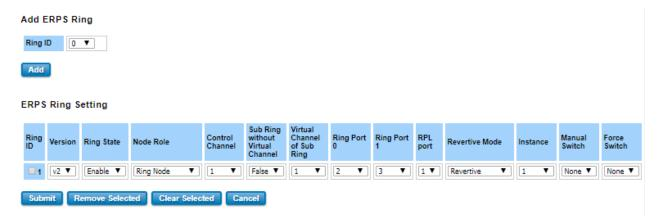
Add ERPS Ring is a section to add the Ring ID of the created Protection group; it must be an integer value between 0 and 31. The maximum numbers of ERPS Protection Groups that can be created are 32. Click the ID of a Protection group to enter the configuration page. After click Add button, one line will be directly created in the ERPS Ring Setting section. The ERPS Ring Setting section is a table that used to set up the ERPS Ring configuration.
