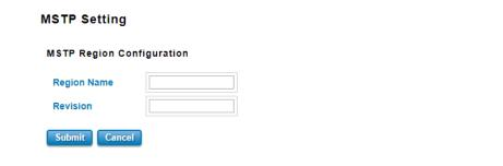
This page allows configure the Region Name and its Revision, mapping the VLAN to Instance and check current MST Instance configuration. The network can be divided virtually to different Regions. The switches within the Region should have the same Region and Revision level.
