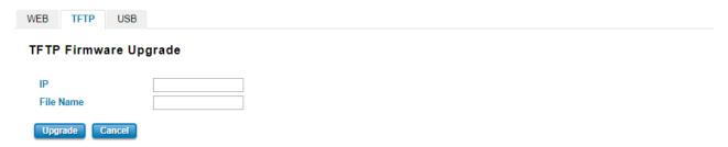
**TFTP Server** mode: In this mode, the switch acts as the TFTP client. Before do so, make sure that TFTP server is ready. Then please type the IP address of TFTP Server and Backup configuration file name. This mode can be used in both CLI and Web UI.
