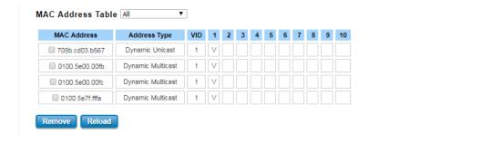
Click on **Remove** to remove the selected static Unicast/Multicast MAC address. Click on **Reload** to refresh the table. New learnt Unicast/Multicast MAC address will be updated to MAC address table.
