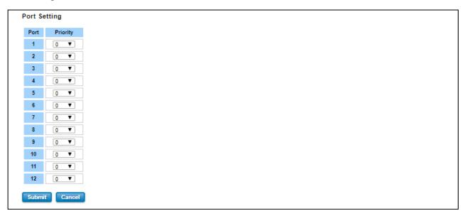
Choose the Queue value of each port, the port then has its default priority. The Queue 7 is the highest port-based queue, 0 is the lowest queue. The traffic injected to the port follows the queue level to be forwarded, but the outgoing traffic does not bring the queue level to next switch. Click the **Submit** button to apply the configuration changes.
