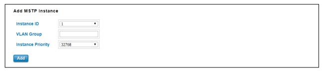
This page allows mapping the VLAN to Instance and assign priority to the instance. Before mapping VLAN to Instance, user should create VLAN and assign the member ports first. Please refer to the VLAN setting page. **After** finish the configuration, click on **Add** to apply user settings.
