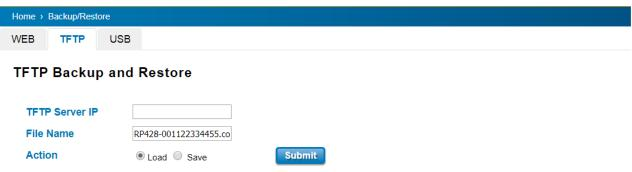
**TFTP Server** mode: In this mode, the switch acts as TFTP client. Before do so, make sure that TFTP server is ready. Then please type the IP address of TFTP Server and Backup configuration file name. This mode can be used in both CLI and Web UI.
