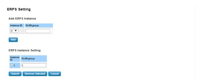
**Add ERPS Instance** is a section for mapping the VLAN to Instance. Before mapping VLAN to Instance, user should create VLAN and assign the member ports first. Please refer to the VLAN setting page.
