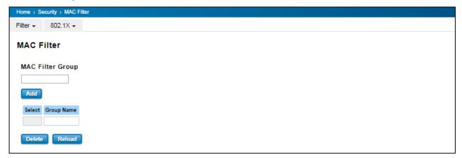
Create a group of MAC Filters by entering a name and clicking the **Add** button to create a new Filter Group. The MAC Filter Group table provides the following information. **Select** the entry and click the **Delete** button then the Filter Group is deleted. Click the **Reload** button to reload the MAC Filter Group table.
