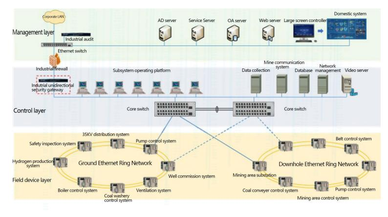
In order to improve the security of the production control system, AVCOMM industrial Unidirectional Security Gateway is deployed between the OT and IT to achieve the physical protection between the automatic industrial ring network and IT. At the same time, whether the collected data and production data can be transmitted to the IT in unidirectional.
