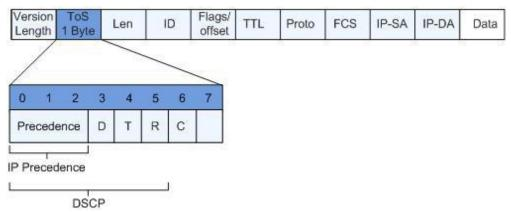
The bits from 0 to 2are the Precedence field, which represents the eight precedence levels of packet transmission. 7,6, ..., 1, and 0 in descending order of precedence. 7 or 6 represents the highest precedence, which is often reserved for routing or updating network control traffic. The user-level applications can only take the precedence from 0 to 5.
