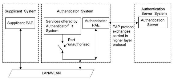
The client is a user terminal device that requests to access the LAN, which shall be authenticated by the device in the LAN. The client shall have the software that supports 802.1X authentication.
