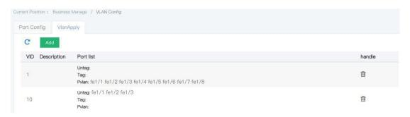
2. Configure the Ethernet ports join the VLAN in the right way, so as to enable VLAN packet message get through. Click the "Networking >VLAN >Port configuration" menu in the navigation tree to enter the interface, tick ports fe1/1, fe1/2, fe1/3, change the value of PVID into 10, click "apply", the interface is shown as the following figure:
