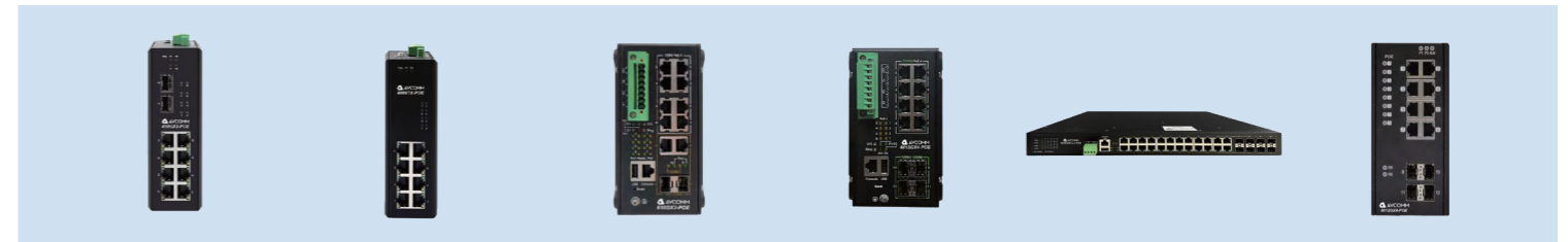
410GX2-PoE 8*10/100 Base-T, 2*1000 Base-X PoE/PoE+ 4008TX-PoE 8*10/100/1000 Base-T PoE/PoE+ 610GX2-PoE 8*10/100 Base-T, 2*1000 Base-X PoE/PoE+ 6012GX4-PoE 8*10/100/1000 Base-T, 4*1000 Base-X PoE/PoE+ 6028GX8-L3-PoE 24*10/100/1000 Base-T, 4*1000 Base-X, 4*Combo PoE/PoE+ 8012GX4-PoE 8*10/100/1000 Base-T, 4*100/1000 Base-X PoE/PoE+
